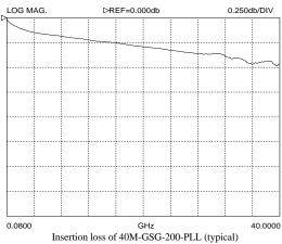
We have shaved another .25 db insertion loss off of our industry standard Model 40A Picoprobe. This probe is recommended for
