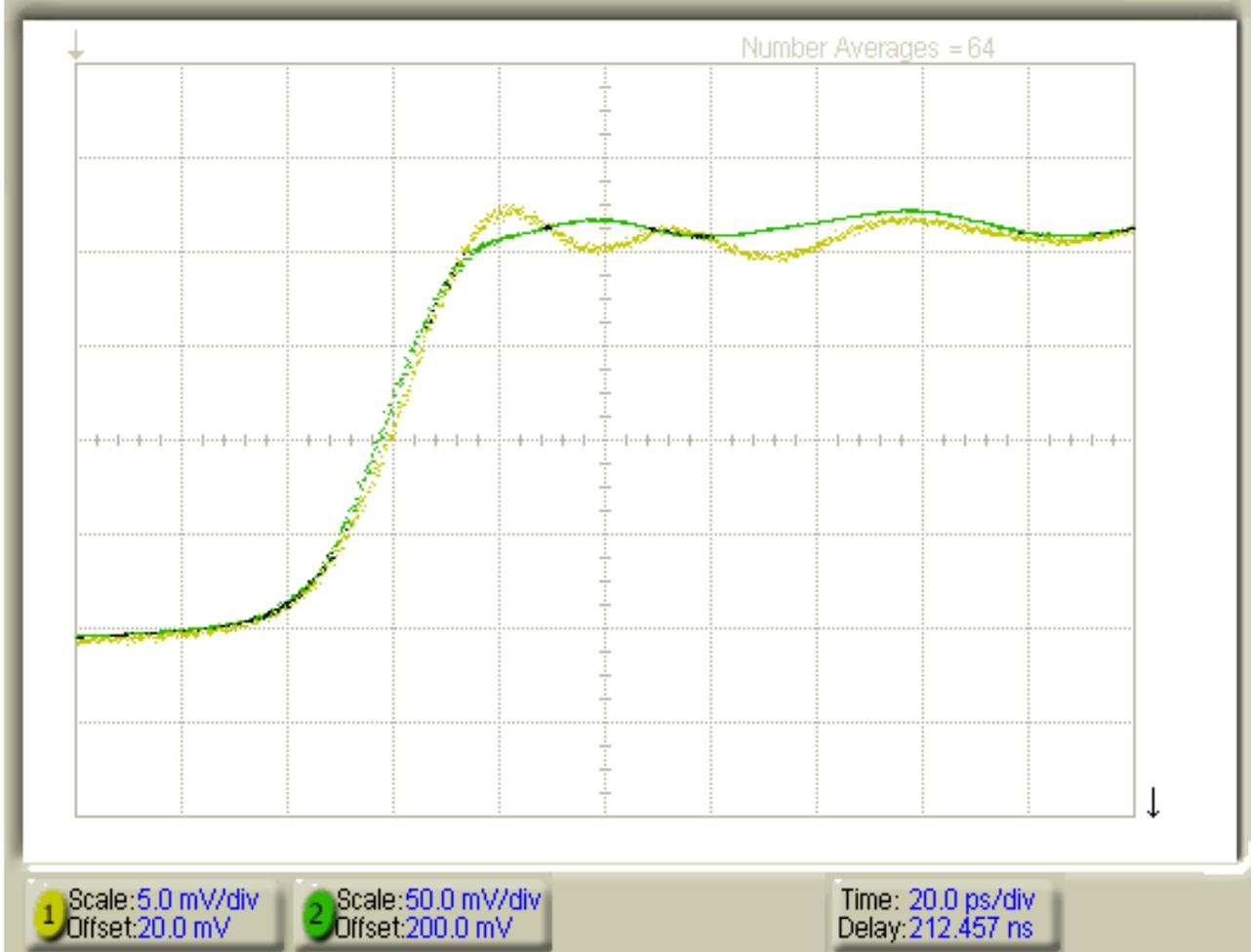
This plot shows the response of the Model 35 Picoprobe to a 0.25 volt, 25 picosecond rise time input pulse. Both the input pulse(Channel 2) and the Model 35 response (Channel 1) are displayed simultaneously on a dual channel 20 GHz sampling oscilloscope. The Model 35 probe tip was contacted to a 50 ohm impedance strip line that carried the input signal. The Model 35 used only a single contact and did not require a short ground connection.
