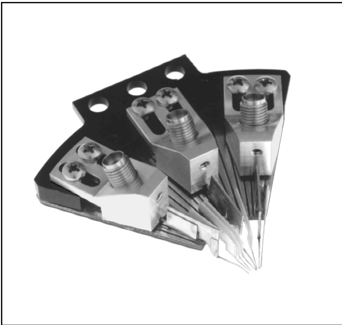
An example of the Picoprobe® Multi-Contact Wedge with three 40 GHz probes and five dc needles.
